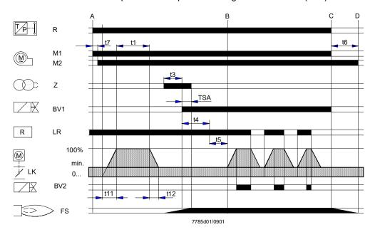
Interrupted pilot burners (burners with pilot burner), controlled and supervised by **LGK16.335** or **LGK16.635**, for example. The other types of burner controls of the LGK16 range program the times safety time (TSA), preignition time (t3), interval (t4) and second safety time (t9) for the pilot burner.
