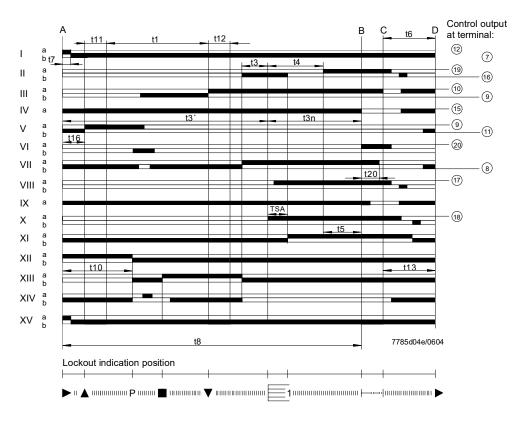
Expanding flame burners (burners without a pilot burner), controlled and supervised by **LOK16** or **LGK16**. Air damper in low-fire position during burner off times (min.).
